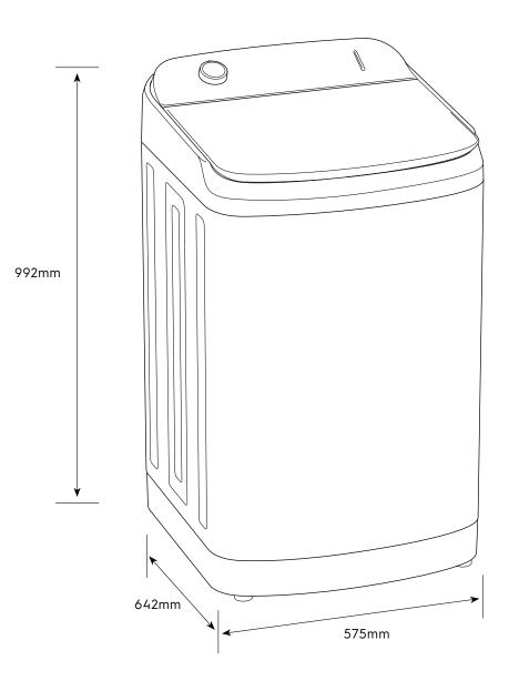
Please note! Dimensions to be used as a guide only. All customers MUST refer to the user manual supplied with the product for detailed installation instructions. © 2022 Electrolux S.E.A PTE. LTD. E\_DIM\_EWT1074M5WA\_Jan22
