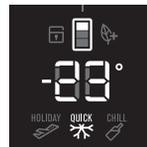
Use the quick freezer mode when you add a large amounts of food to the freezer compartment. The freezer compartment temperature will show -23°C. (This temperature cannot be changed while pressing the "Modes" button to select quick freeze will now operate for 90 minutes then switch to normal operation.)
