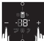
1. Press left "<" arrow button to make the freezer colder in 1°C steps.
