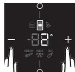
1. Press left "<" arrow button to make the middle colder in 1°C steps.
