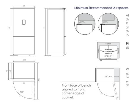
Allow a minimum of 10mm clearance above the hinge cover.
