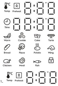
Temperature display, from 40°C-230°C, when In preheat phase, the "Preheat Indicator" wlll blinking.
