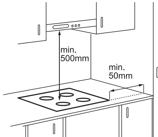
\*The clearance must meet or exceed the minimum recommended for both the rangehood and cooktop. Refer to the rangehood installation manual.
