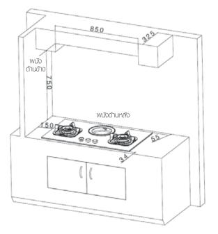
\*To combustible surface (dimension is not relevant if the adjacent surface is non-combustible).
