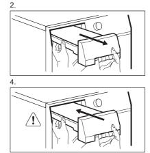
You can use the water from the water container as an alternative to distilled water (e.g. for steam ironing). Before you use the water, remove dirt residues with a filter.
