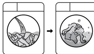
After press Start/Pause touchpad, the machine will start add water to the washing drum, which will start to rotate slowly to dissolve detergent and evenly distribute cloths.
