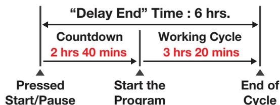
After select Delay End time, press Start/Pause touchpad to start the program. Machine will then countdown and update time on the display every hours until it reaches the starting point of the wash cycle.
