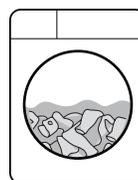
The machine will enter the process of soaking, The washing drum will stop and rotate once in a while in order to redistribute cloths.
